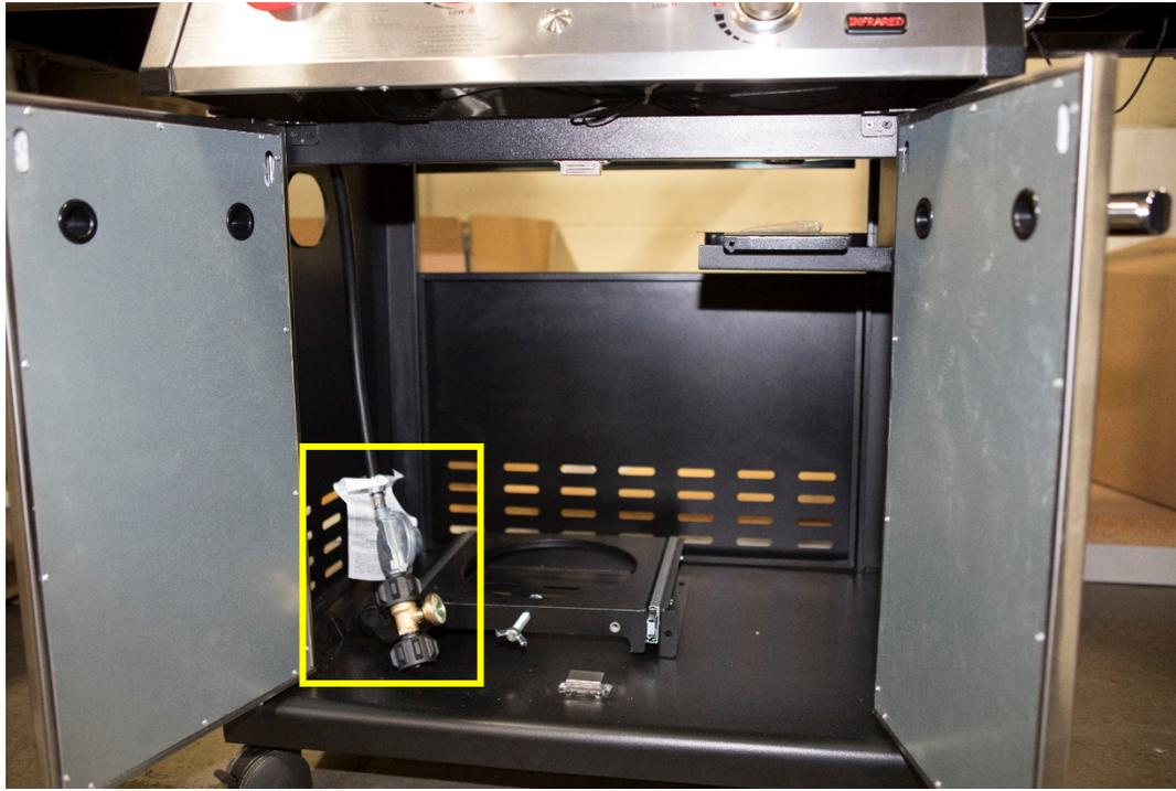
**Recalled grill - fuel line not mounted to side of grill AND fuel gauge on regulator assembly**
